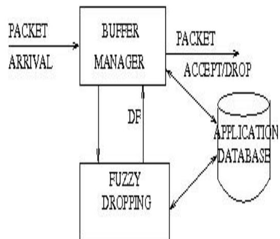
Fig.1. Fuzzy Based Packet Dropping Scheme
