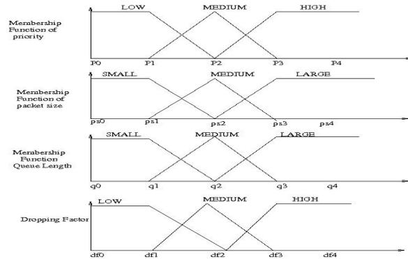
Fig. 3. Membership function for input and output linguistic parameters
