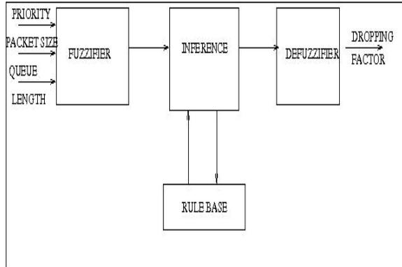
Fig.2. Fuzzy Packet Dropping Probability Computation
